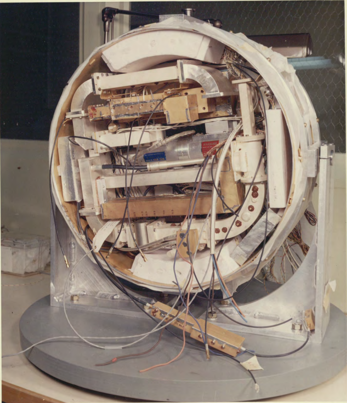
Components in canister which is to be placed inside the satellite shell. Photographed during construction of one of the actual "fly" models.
